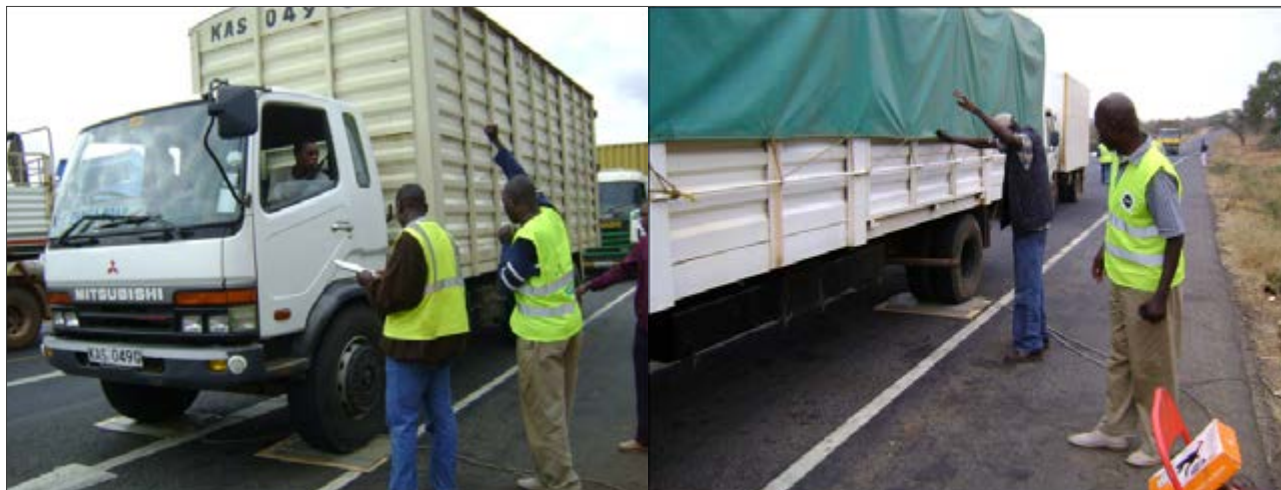
Figure 7.4 Vehicle's Front and Rear Wheels Adequately Accommodated by the Weigh Pad
